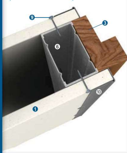
Installation of door jamb details (with boxed steel stud)
